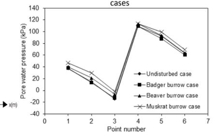
Figure 7. The change of pore water pressures with respect to different cases
