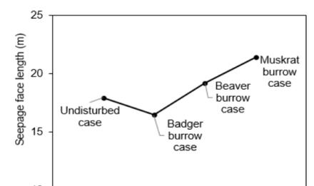
Figure 5. Seepage face lengths for four different cases
