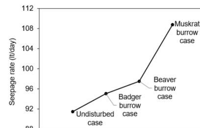
Figure 4. Seepage rates passing through the centerline for four different cases
